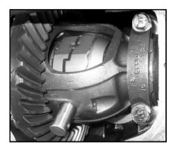
9.) Check the Center Gap Measurement: Use your caliper or feeler gauges to measure the gap between the two cam gears with the locker teeth engaged. This is an installation check to see if the thrust washers were installed or to see if the differential case is within average machining tolerances or if it has become worn. If the gap is out of specifications, please contact Customer Support: Info@TorqMasters.com
