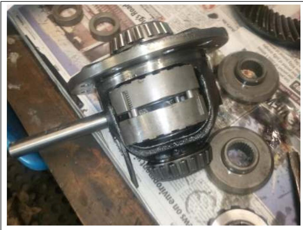
Checking to see if the locker cleared the carrier sometimes one needs to grind a small amount
