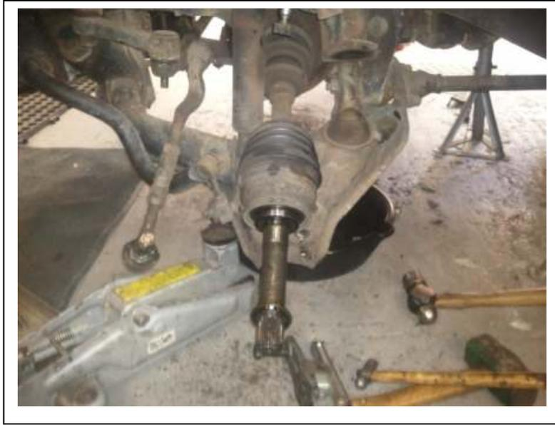
Finally the knuckle removed now you need to give a strong pull to release the drive shaft be careful if your vehicle is on a jack, do not let the splines of the shafts damage the seals
