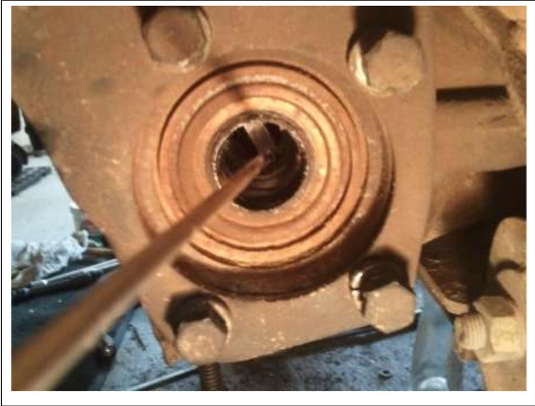
Use a long thin screw driver to line up the splines from outside the diff
