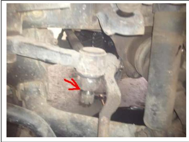
Remove the steering control arm completely
