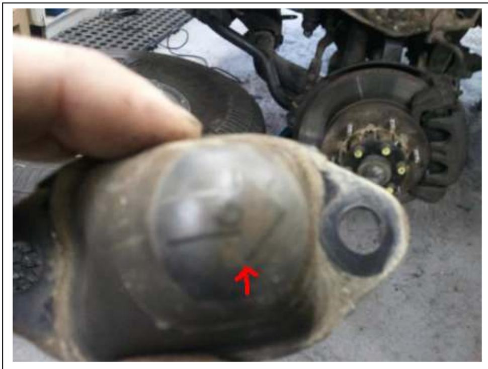
This is the bump stop from the top control arm I removed them as I did this job on my own and was not able to get the bottom and top control arms to connect, with the bump stops removed I could manipulate the two together after loosening the torsion bars this took a huge effort and I battled for ages on this part I never knew I could swear so much, note the arrow on the bump stop it faces towards the engine
