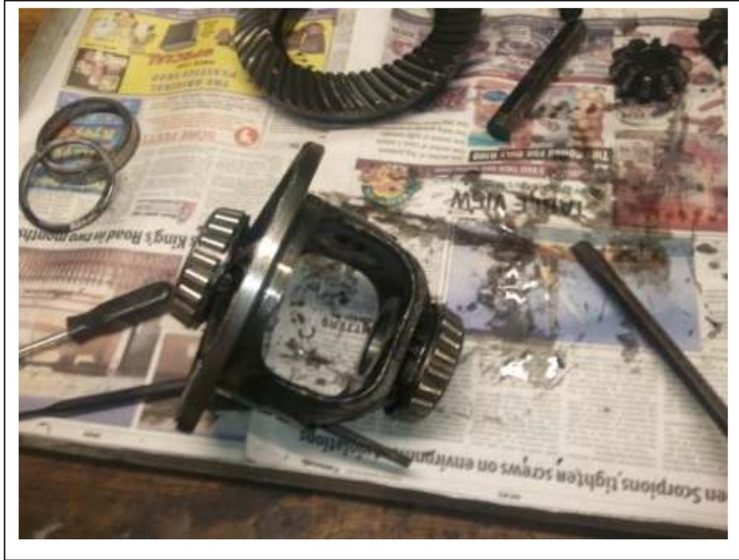
Empty Carrier keep the original shims from the spider gears to use with lokker
