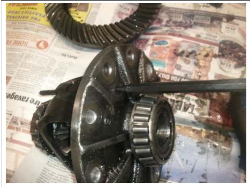
After removing the crown wheel knock out the pin do not remove the pin completely
