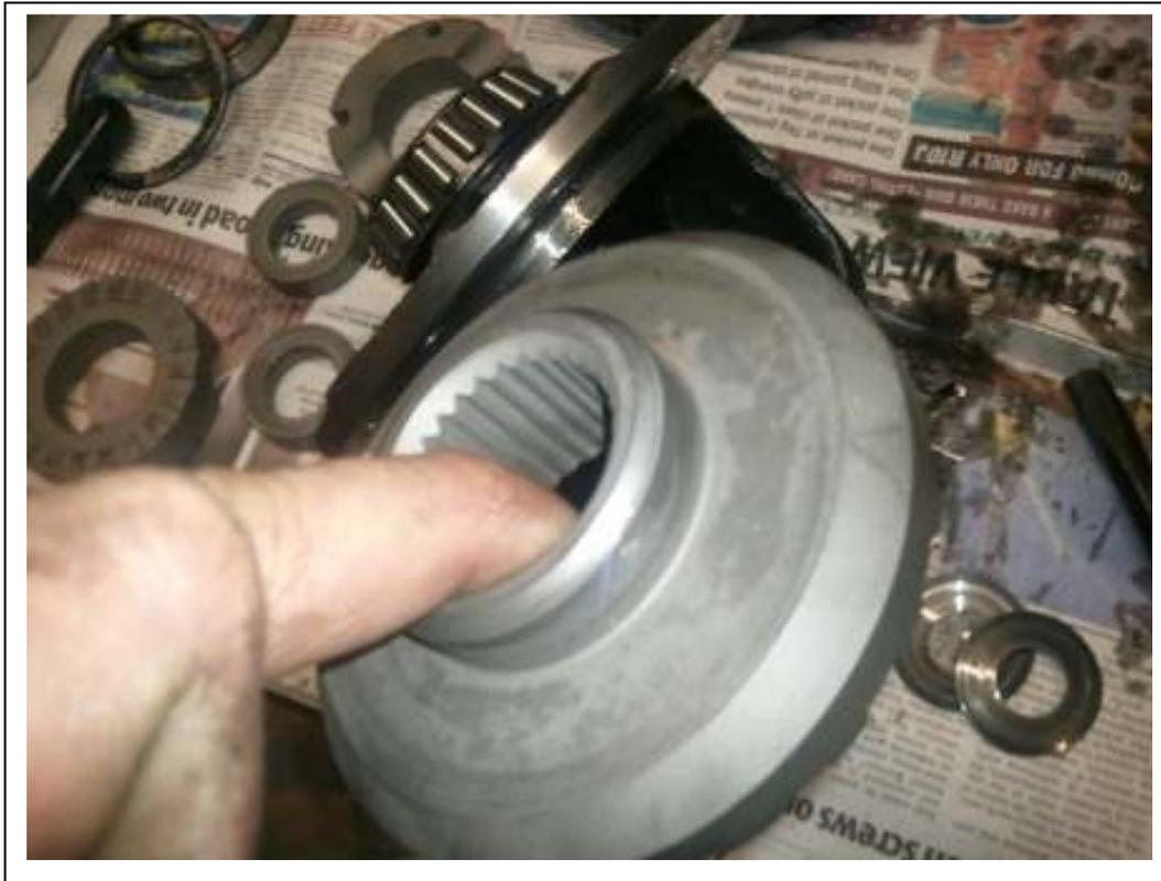
Grease all components before installation
