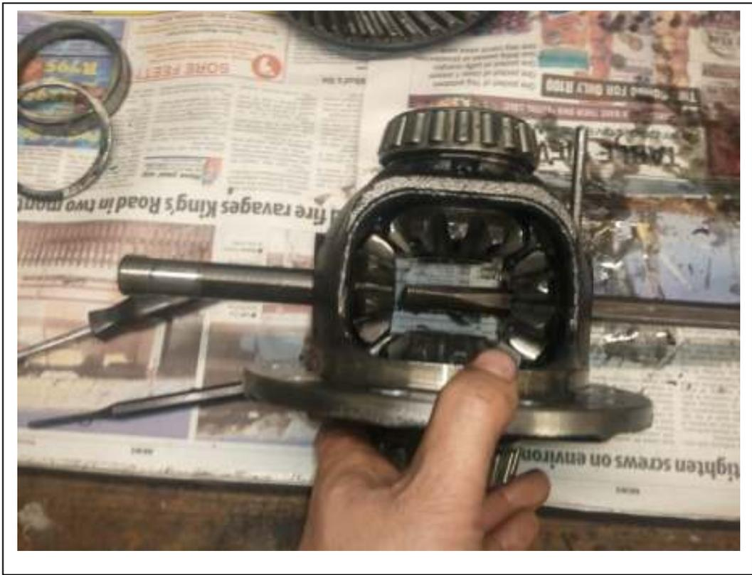
Now you can remove the shaft in order to remove the spider gears
